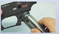
Once the motor is in-place, insert the Motor Fixing Pins. If the pin do not fit in smoothly and tapping/hammering is required, make sure the motor is properly and evenly supported first. A piece of board under the motor to distribute the pressure would work. This is important because the motor is a structural part of the PTW, and it must not be deformed.
